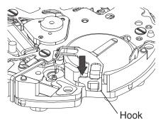
(3) Winding stem ·How to remove
