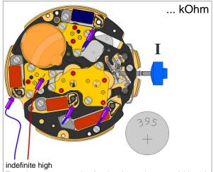
The resistance between each coil and +pole must be measured (electronic module must be removed)
