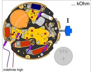
The resistance between each coil and +pole must be measured (electronic module must be removed)
