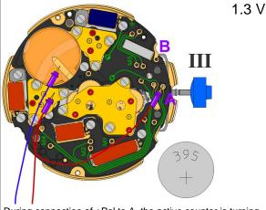
During connection of +Pol to A, the active counter is turning. Reduced the supply voltage to 1.3V to check the proper function of the counter. If the power supply is disconnected, the control mode must be starded again section 1. 1. Activation of control mode (pos III)
