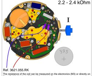
The resistance of the coil can be measured on the electronics (M3) or directly on the coils (electronic module must be removed).
