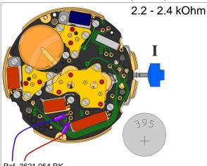
Resistance of the coil: motor 3 (counter)
