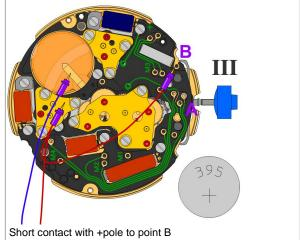
Change of active counter: M2-M3-M4-M2-M3- .After a timout of approx. 30 seconds since last contact, the control mode will be terminated.
