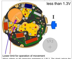
Adjust voltage on the measuring eqipement to 1.55 V. The slowly reduce the tension until the movement stops
