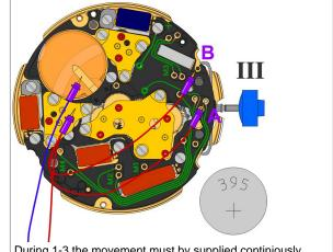
During 1-3 the movement must by supplied continiously Connect points A + B simultaneous for min. 2 seconds to the +Pol. Do not interrupt the supply voltage - stem pos III)
