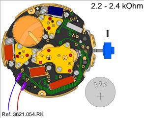
The resistance of the coil can be measured on the electronics (M4) or directly on the coils (electronic module must be removed).
