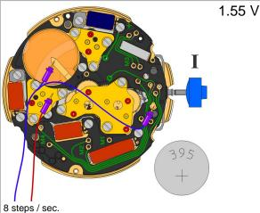
To activate this test mode, the corresponding test point must be connected to the -Pole
