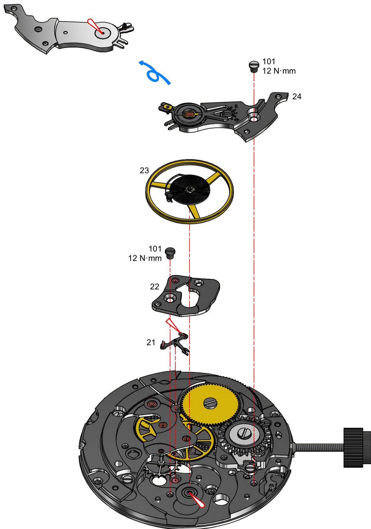
**Montage mouvement – Werkmontage – Assembling of the movement
