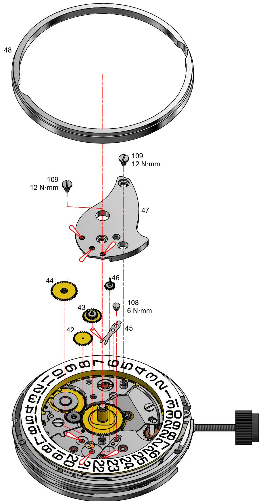
**Montage mouvement – Werkmontage – Assembling of the movement
